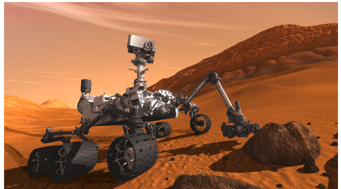
The Mars rover Curiosity is equipped with a LIBS spectrum analyzer Image courtesy NASA/JPL-Caltech
